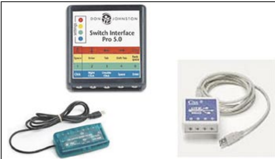
Figure 8: A switch interface was necessary since a portable computer was used to address possible use of dynamic display. Shown here are the Don Johnston Switch Interface Pro 5.0, Crick USB Switch Interface and Wivik USB Switch Adaptor Box from Prentke Romich Company.
