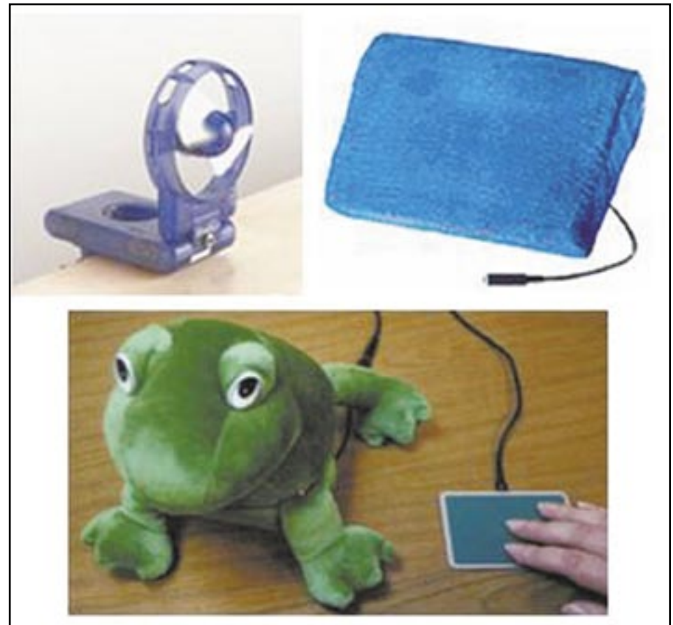
Figure 6: Switch activated devices were included to assess cause and effect, as well as serving as positive reinforcement during the assessment process.
