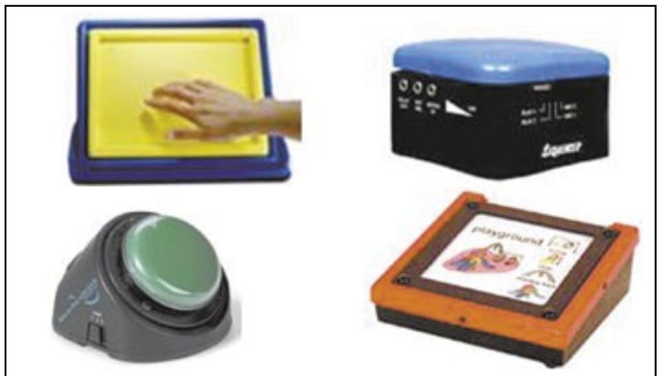
Figure 3: A variety of sequencers were available in the different Assistive Technology labs. Included were step communicators from Enabling Devices, Adaptations, AbleNet and AMDI. These devices could be used for assessing potential for single message use as well as communication exchanges.
