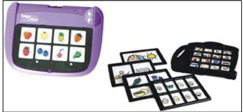
Figure 4: The versatility of a static display voice output device that has the option of being configured into one or multiple messages was considered essential for a basic diagnostic kit. Pictured here are the SuperTalker by AbleNet and the 7 Level Communication Builder by Enabling Devices.
